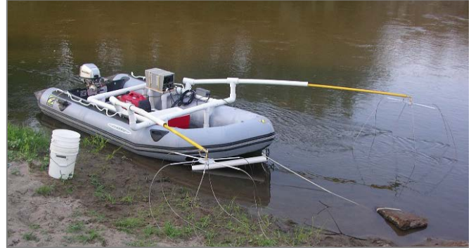
Figure 2-9 Photograph of Boat-Mounted Electrofishing Apparatus
