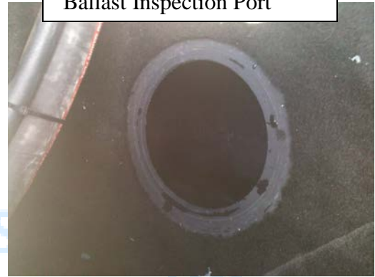
2014 Centurion Enzo 244 Ballast Inspection Port
