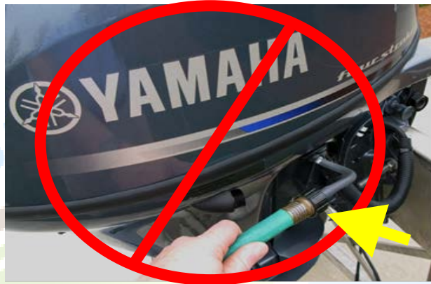
Improper Flushing Technique for Outboards
